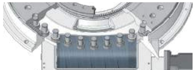
This cooling carousel at one of Cirex's casting stations in the Netherlands has a diameter of 10 metres and weighs 30 tonnes. It is driven by a CR. A special bearing has been fitted to handle the high tilting moment as a result of the uneven load.
