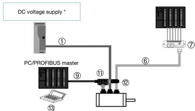
\* voltage supply: STP 24 VDC, BLM/BLM high power 24-48 VDC
