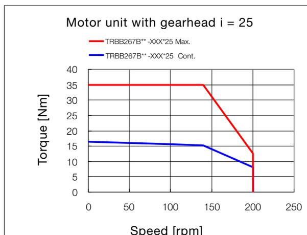
External conditions: 48 VDC supply voltage at ambient temperature of 40°C.
