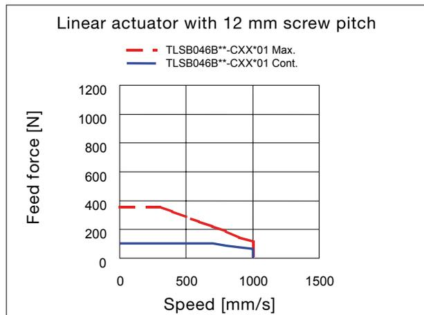
External conditions: 48 VDC supply voltage at ambient temperature of 40°C.
