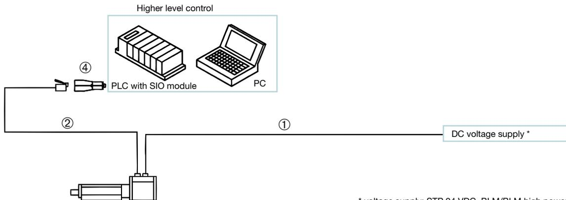
\* voltage supply: STP 24 VDC, BLM/BLM high power 24-48 VDC
