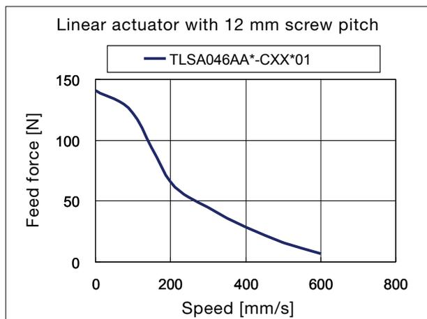
External conditions: 24 VDC supply voltage at ambient temperature of 40°C.
