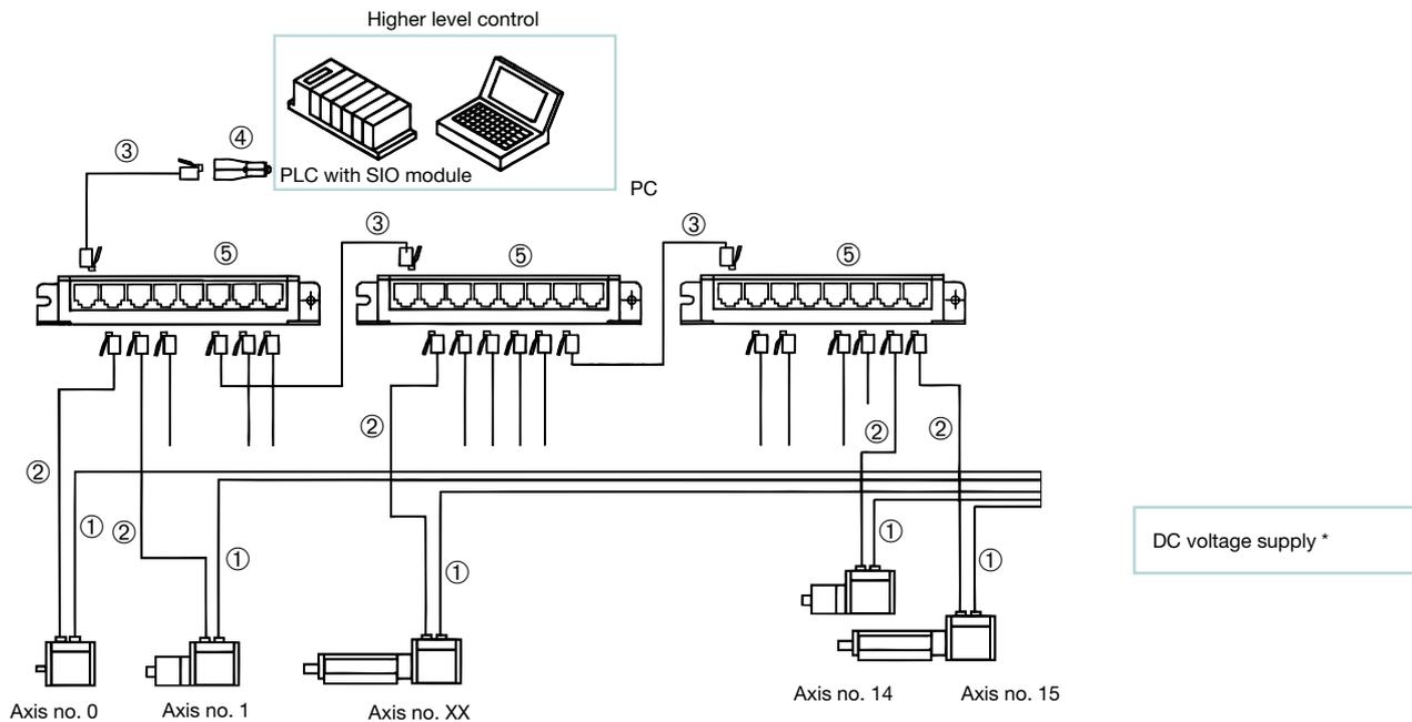
\* voltage supply: STP 24 VDC, BLM/BLM high power 24-48 VDC
